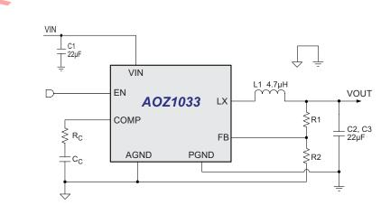
Figure 1. 3.3V 3A Synchronous Buck Regulator
