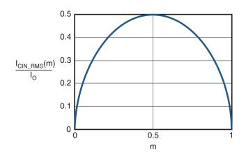
Figure 2. I<sub>CIN</sub> vs. Voltage Conversion Ratio
